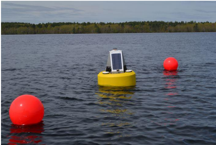
Figure 5: NexSens water quality monitoring buoy. This photo is from Portland Water District and shows the system deployed on Sebago Lake.
