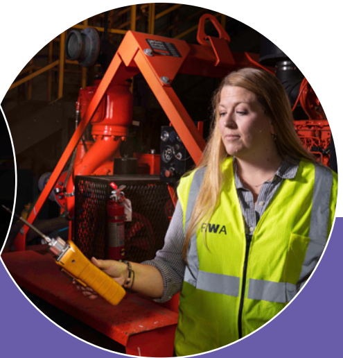
Amanda Schenkle, Manager of Safety and Risk , uses a photoionization detector to identify any volatile organic compounds in the air. Among Amanda's many duties, she works to ensure the health and safety of our 270 employees.
