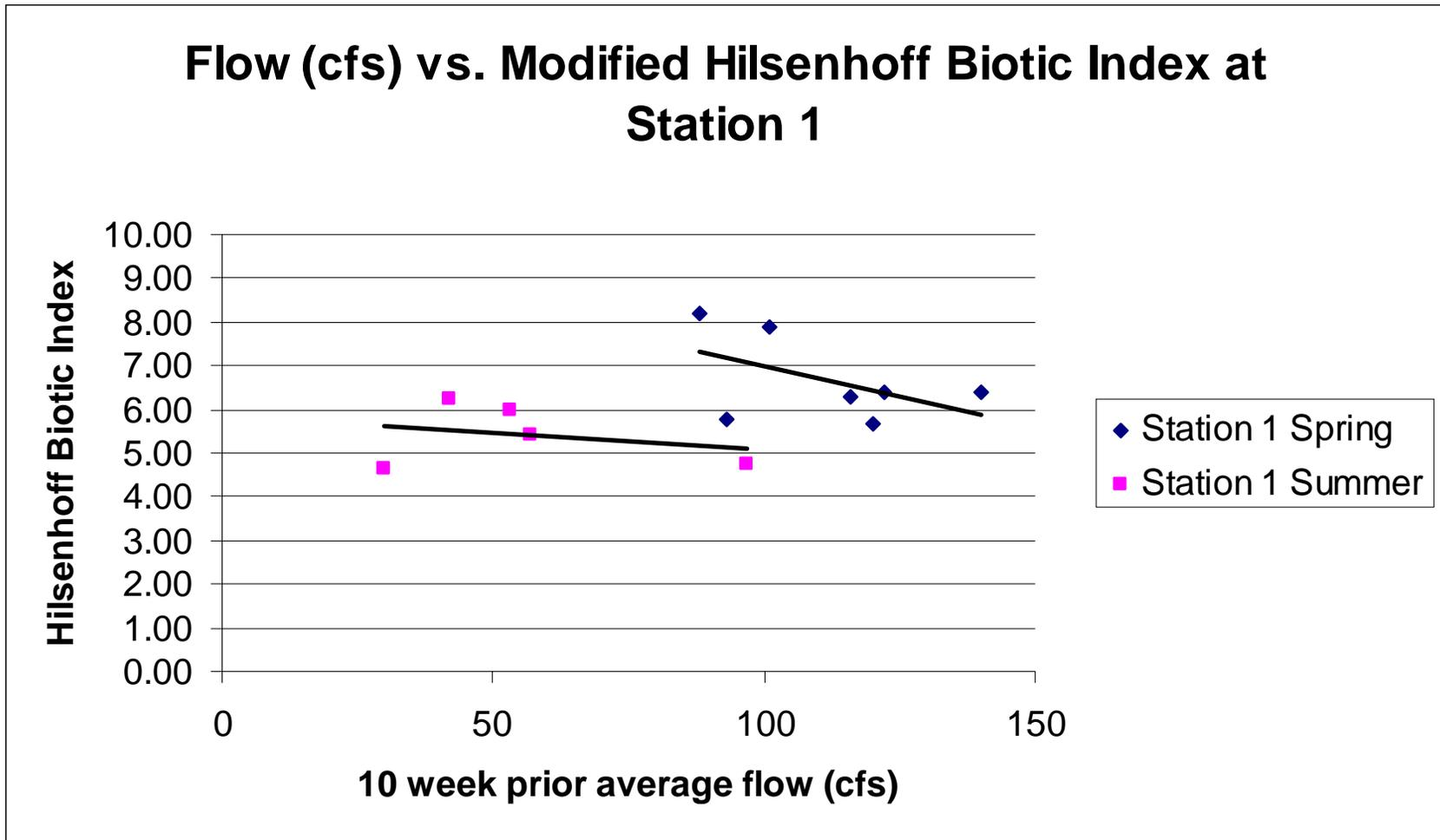
Figure 11. A graph of HBI values vs. average flow for 10 weeks prior to macroinvertebrate sampling for 2000-2006 at station 1.
